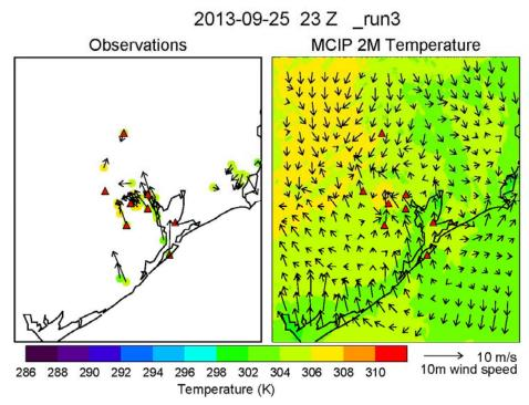
Figure 2. Observed (left) and WRF diagnosed (right) 2 m temperature and 10 m wind velocity at 23 UTC 25 September 2013 from the new 1 km WRF simulation. Strength of WRF simulated bay and sea breezes in agreement with observations.
