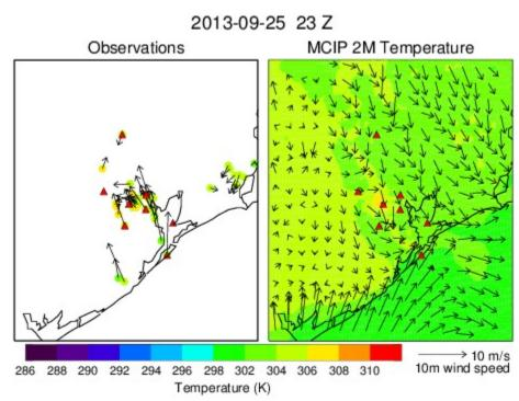
Figure 1. Observed (left) and WRF diagnosed (right) 2 m temperature and 10 m wind velocity at 22 UTC 25 September 2013 from the original 4 km WRF simulation. WRF simulated weaker sea and bay breezes than observed.
